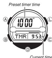
The watch includes a number of different preset times that you can select for the countdown start times. An alarm sounds when the countdown reaches zero.
